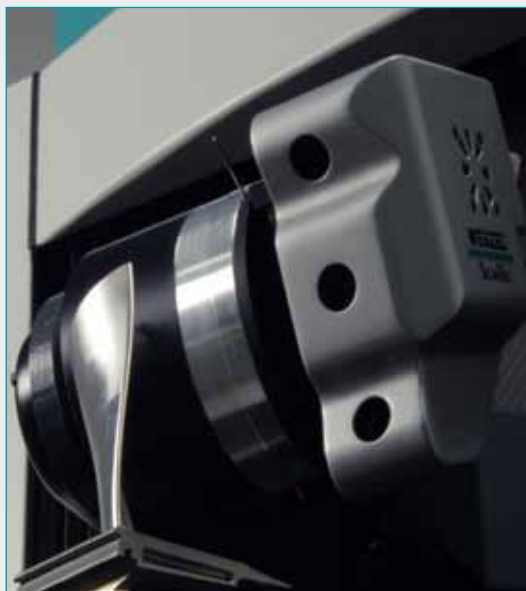
Measurement of a turbine blade
